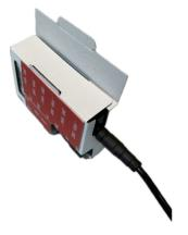
8. Check the device alignment: the USB connector, the display, the start and stop buttons, and the barcode should be visible in the folded box. Note how the probe connector of the Saga-P device slides into the oval cutout. Placing a Saga device into the box leaves the oval cutout empty.
